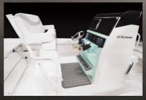
**LEAN POST BACKREST:** Leaning post features thigh rise bolsters and arm rests for multiple seating configurations. Custom color matching helm comes standard with hydraulic tilt steering, fatigue reducing EVA padded foot rest and cockpit sole.
