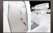
**OVERSIZED CONSOLE:** Features a full width and height side entry door. Large enough to add a portable toilet or serve as a changing room. Custom breaker panel and large access panel can also be found in the console.
